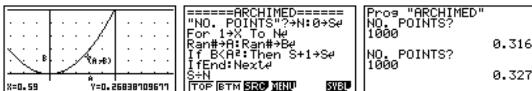
Figure 12. A Monte Carlo determination of the area under the curve y = x^2
