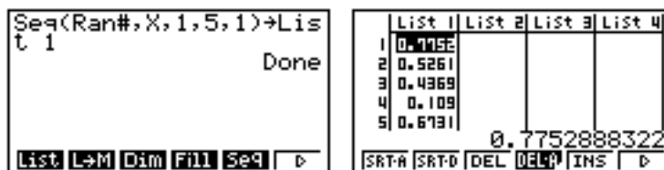
Figure 3. Using a sequence command to generate a set of five random numbers on (0,1)
