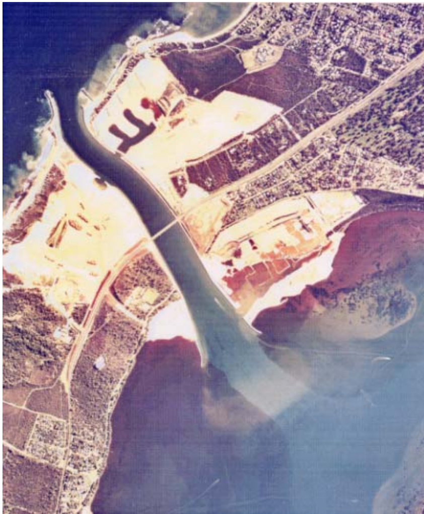
Figure 4.1. Dawesville Channel in July 1994. This photograph was taken at high tide. Clearly visible is the salt water intrusion from the channel.
