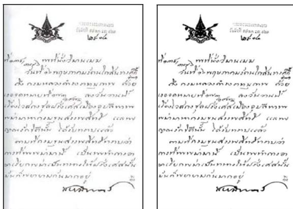
Figure 2. The image on the left is the scanned image and the one on the right is the processed binary image from Otsu's Algorithm
