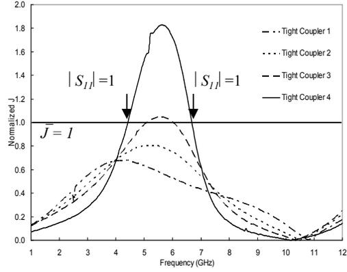
**Figure 2: Frequency-Dispersive Behavior of Normalized  $J$ -Susceptance of a PCML with varying  $w_o$**
