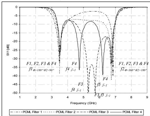
**Figure 6: Returns Loss Responses of PCML Broadband Filter with various  $w_o$  and  $w_l$**
