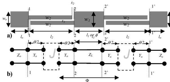
Figure 4: A PCML Broadband Bandpass Structure (a) Configuration, (b) Equivalent  $J$ -inverter.
