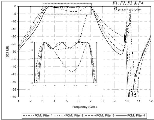
**Figure 5: Insertion Loss Responses of PCML Broadband Filter with various  $w_o$  and  $w_l$**
