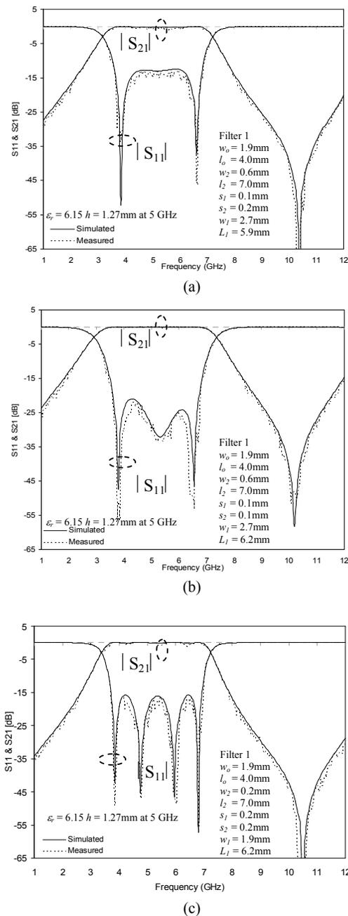
**Figure 7: Simulated and measured results of the three PCML broadband bandpass filters.**
