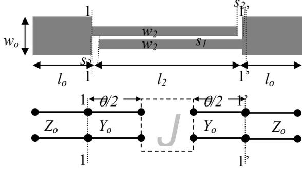
**Figure 1: A PCML Structure (a) Configuration, (b) Equivalent  $J$ -inverter.**
