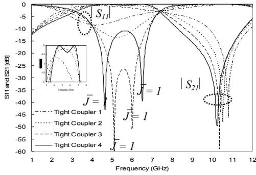
Figure 3: Insertion and Return Losses of PCML Structure with Varying  $w_o$ .
