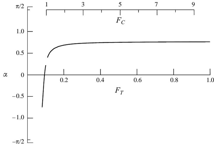
FIGURE 5. The variation of the entry angle  $\alpha$  with the withdrawal Froude number  $F_T$ , for the case  $\delta_2 = 0.25$ ,  $D = 0.95$ . Solutions to the right of this figure have been obtained with  $\lambda_2 = 0.5$ . The combination Froude number  $F_C$  is also indicated.
