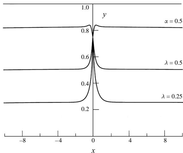
FIGURE 8. Three interface profiles for  $\delta_2 = 0.75$ ,  $D = 0.95$ . The bottom solution has been obtained with  $F_T = 0.4$  and  $\lambda_2 = 0.25$ , and the middle surface represents  $F_T = 0.4$  and  $\lambda_2 = 0.5$ . In the top solution, the entry angle was set to the value  $\alpha = 0.5$ , and both the Froude number and the upstream depth were determined from the numerical solution.
