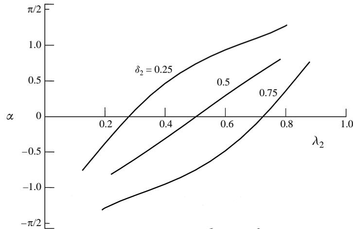
FIGURE 2. The variation of the entry angle  $\alpha$  with the upstream interface height  $\lambda_2$ , for the case  $D = 0.95$ ,  $F_T = 0.5$ . Three sets of results are shown, for sink elevations  $\delta_2 = 0.25$ ,  $0.5$  and  $0.75$ .
