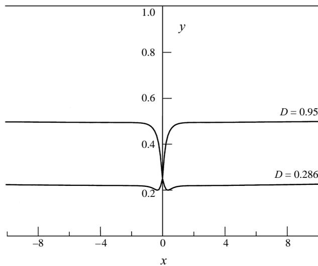
FIGURE 10. Two interface profiles for  $\delta_2 = 0.25$ ,  $F_T = 0.5$ . The top solution has been obtained with  $D = 0.95$  and  $\lambda_2 = 0.5$ . In the bottom solution, the density ratio is  $D = 0.286$ , and both the entry angle and the upstream depth were determined from the numerical solution.
