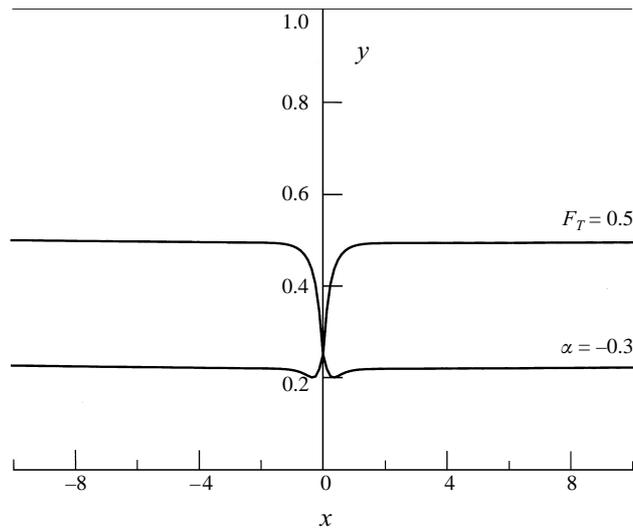
FIGURE 6. Two interface profiles for  $\delta_2 = 0.25$ ,  $D = 0.95$ . The top solution has been obtained with  $F_T = 0.5$  and  $\lambda_2 = 0.5$ . In the bottom solution, the entry angle was set to the value  $\alpha = -0.3$ , and both the Froude number and the upstream depth were determined from the numerical solution.
