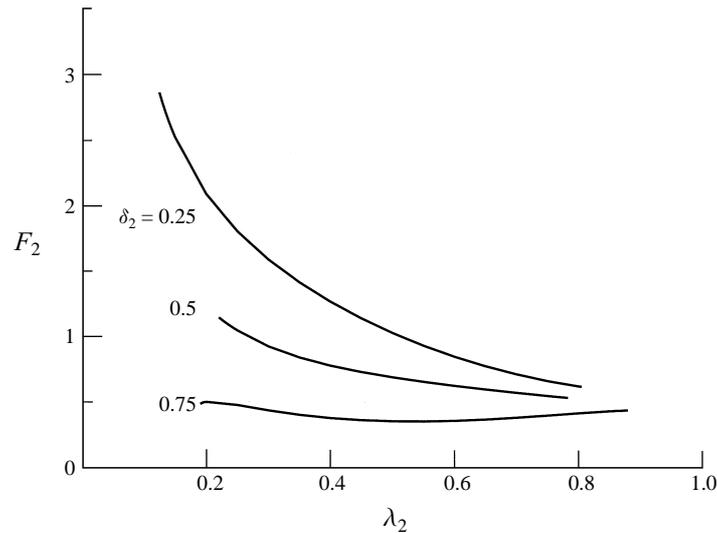
FIGURE 3. The variation of the Froude number  $F_2$  in the lower layer with the upstream interface height  $\lambda_2$ , for the case  $D = 0.95$ ,  $F_T = 0.5$ . Three sets of results are shown, for sink elevations  $\delta_2 = 0.25$ ,  $0.5$  and  $0.75$ .
