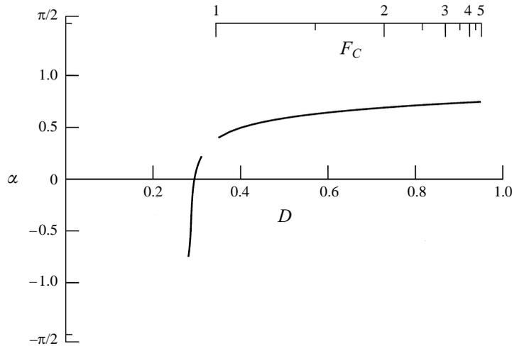
FIGURE 9. The variation of the entry angle  $\alpha$  with the density ratio  $D$ , for the case  $\delta_2 = 0.25$ ,  $F_T = 0.5$ . Solutions to the right of this figure have been obtained with  $\lambda_2 = 0.5$ . The combination Froude number  $F_C$  is also indicated.
