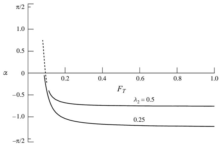
FIGURE 7. The variation of the entry angle  $\alpha$  with the withdrawal Froude number  $F_T$ , for the case  $\delta_2 = 0.75$ ,  $D = 0.95$ . Two sets of supercritical results are shown, for upstream interface heights  $\lambda_2 = 0.25$  and  $0.5$ . The isolated subcritical branch of solutions (sketched with a dashed line) is a branch of solutions for which  $\lambda_2$  is determined as part of the solution.
