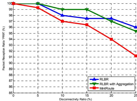
Figure 4. Average Packet Reception vs. Link Failure Ratio
