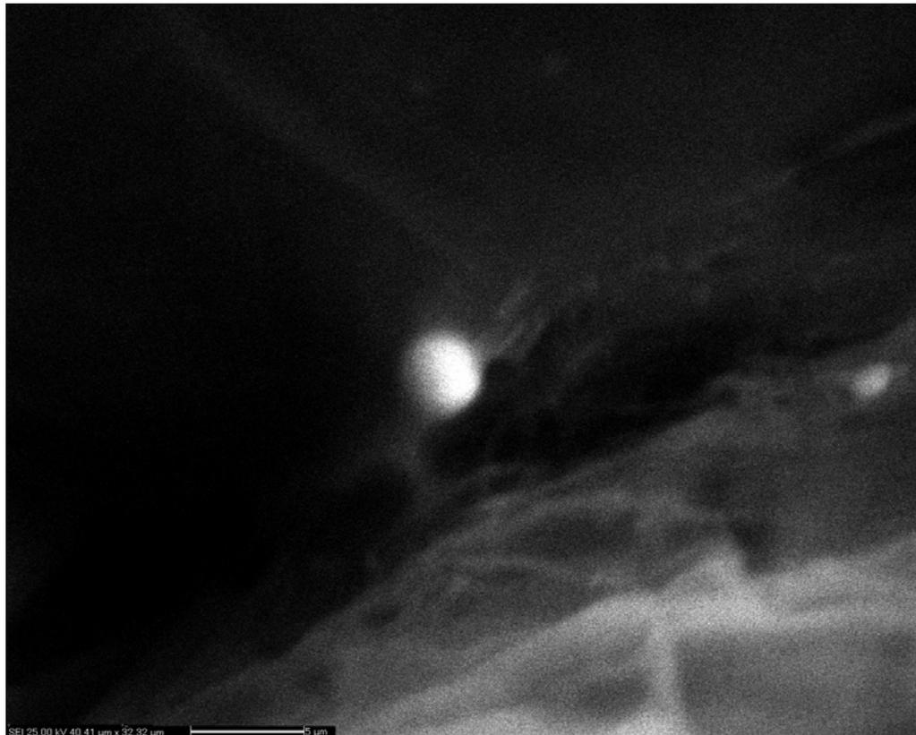
IMAGE 2—The secondary electron image of the BaAl particle found in the arson and explosives room. Note its very small size (<10  $\mu$ m) and spherical shape.
