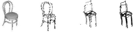
Figure 5: From left to right are 3D model, noised 3D model, point-based 3D sketch and edge-based 3D sketch.
