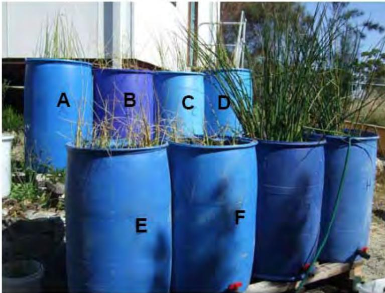
Figure 2. Experimental setup. A,C – VF. D – FWS/VF (woodchips). E,F - FWS/VF (ethanol); B – faulty, not used.
