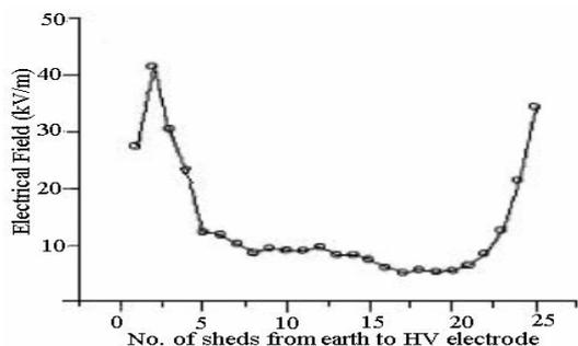
Fig. 14b. Electrical field distribution of contaminated insulator
