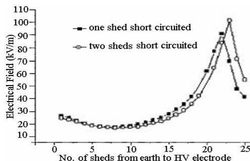
Fig. 15. Electrical field distribution of contaminated insulator with one or two sheds short circuited
