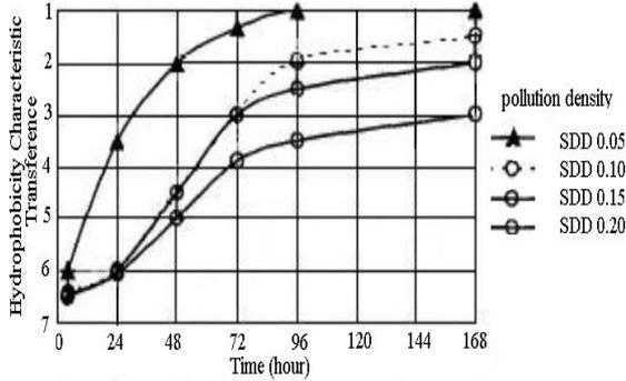
Fig. 9. HC transference of polluted silicone rubber insulators for different pollution densities vs. time lapse after contamination
