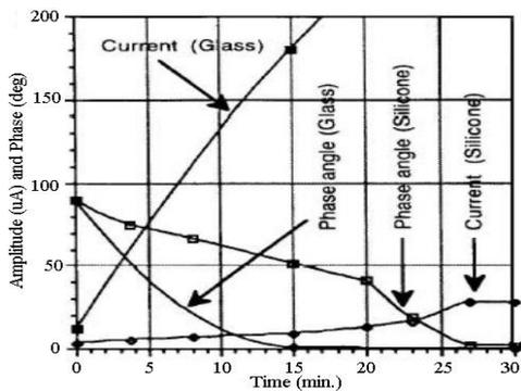
Fig. 6. Bode diagram of LC of two different insulators
