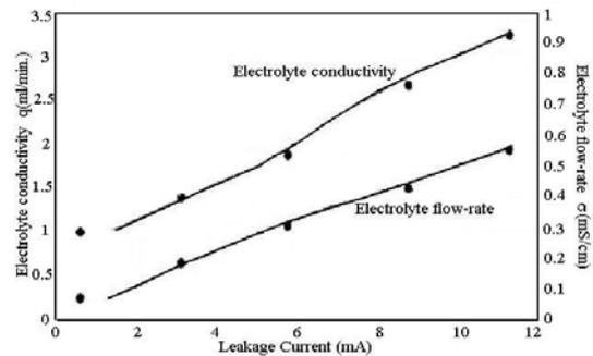
Fig. 3. LC relativity to electrolyte flow-rate and conductivity
