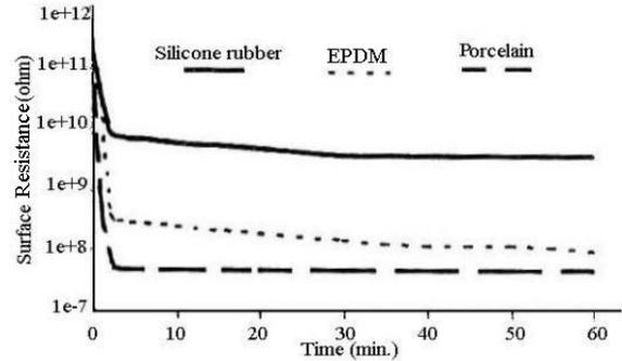
Fig. 7a. SR measurement of three different insulators for spray wetting test
