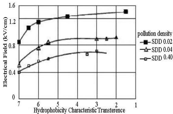
Fig. 10. Electrical field causing flashover for different pollution densities vs. HC levels
