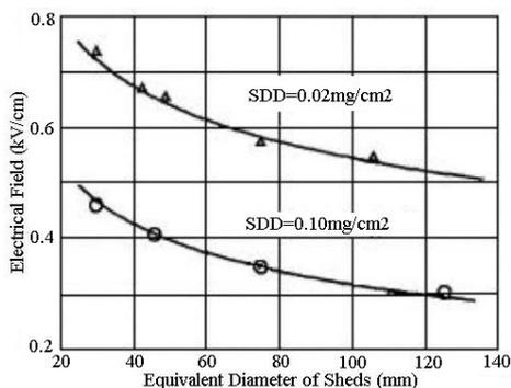
Fig. 13. Electrical field causing flashover for different pollution densities vs. shed diameters of composite insulator
