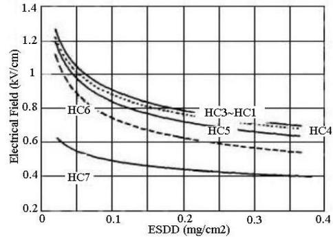
Fig. 11. Electrical field causing flashover for different ESDD on the surface for different HC levels
