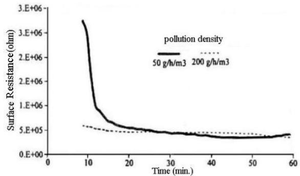
Fig. 8. SR measurement of two different insulators for fog wetting test with different pollution densities
