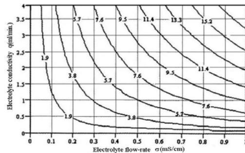
Fig. 4: Electrolyte flow-rate and conductivity relations for different LC levels
