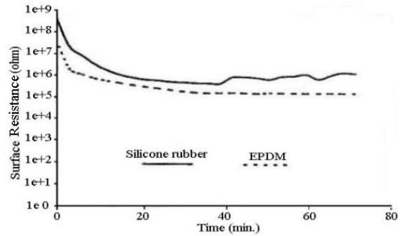
Fig. 7b. SR measurement of two different insulators for fog wetting test
