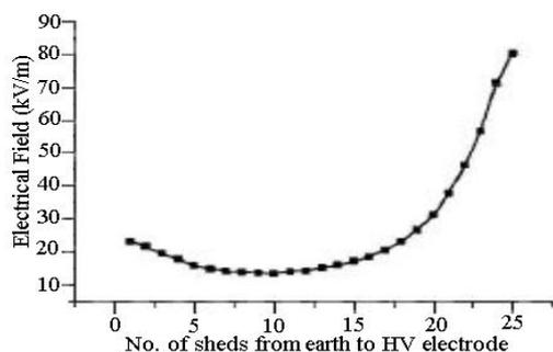
Fig. 14a. Electrical field distribution of clean insulator
