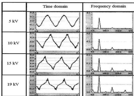
Fig. 2. LC waveforms of silicone rubber insulator in time and frequency domains one day lapse after contamination for different applied voltages
