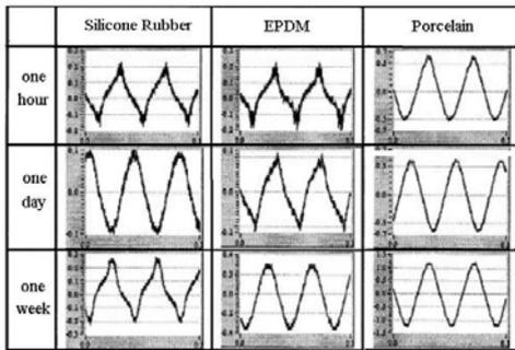
Fig. 1. LC waveform of three different insulators for different time lapses after contamination for applied constant 5 kV
