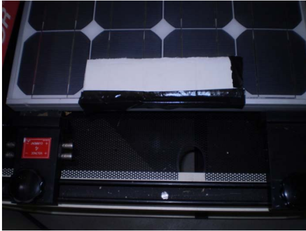
Figure 49 - BP275F Module with the Two Central Cells at the Left Corner half shaded
