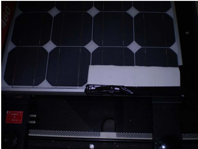
Figure 45 - BP275F Module With Two Cells at the Front of the Tray and the Left Corner Half Shaded
