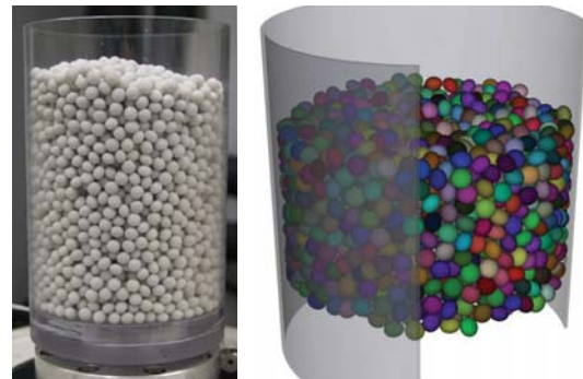
FIGURE 1. (left) Loose jammed packings of frictional ellipsoidal gypsum particles ( 5.3 \times 6.6 \times 6.6 mm) produced with a 3D printer are prepared in a cylindrical container with a diameter of 104 mm. By periodic vertical tapping of the container, the packing can be further compactified. With this method packings of different packing fraction can be prepared by variation of the number of taps. (right) Detected particles after imaging by X-Ray tomography and reconstruction.
