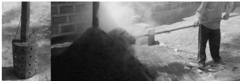
Figure 1. The conventional “open-type” rice husk carbonizer (left) and in operation (right).
