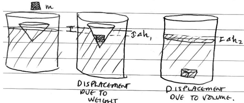
Figure 2. How to use buoyancy to find the density of an irregularly shaped object
