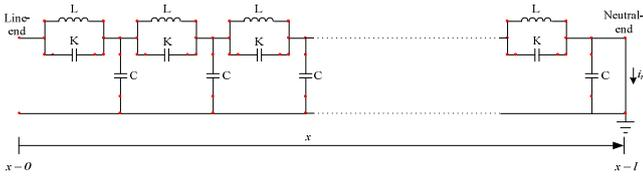
Fig. 2. Impedance measurement in transformer ladder network.
