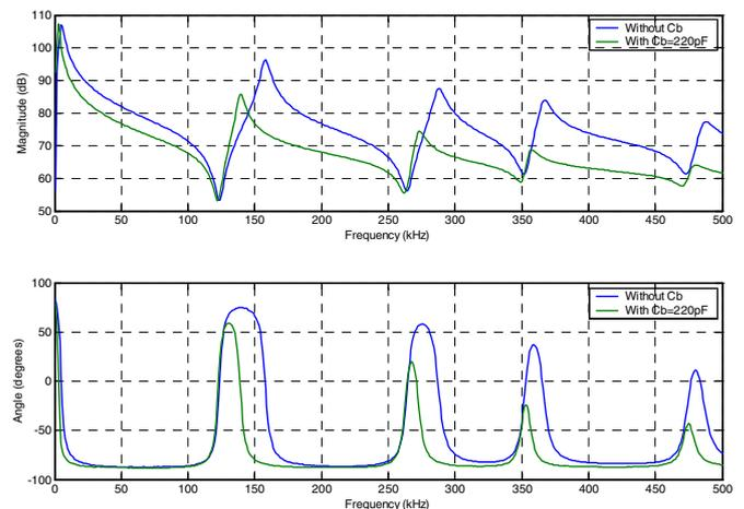
Fig. 5. Measured impedance of the 11kV winding with and without 220pF bushing capacitance  $C_b$ .
