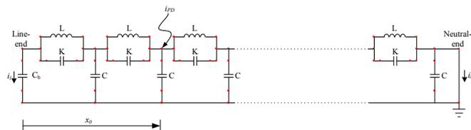
Fig. 1. Ladder network of a transformer at high frequencies.
