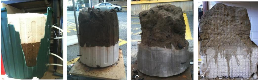
FIG. 11. Results of biocementation of a 3-D sample of 80 L of sandy soil topped with about 32 L of fine silica sand. (a: cemented sample in cylinder container, b: dismantled cemented sample, c: cemented sample was hosed with tap water, d: vertical cross section along the longitudinal centerline.
