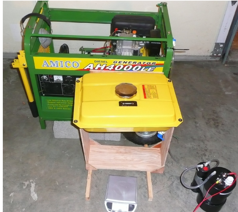
Figure 2: Generator/weight measurement set up
