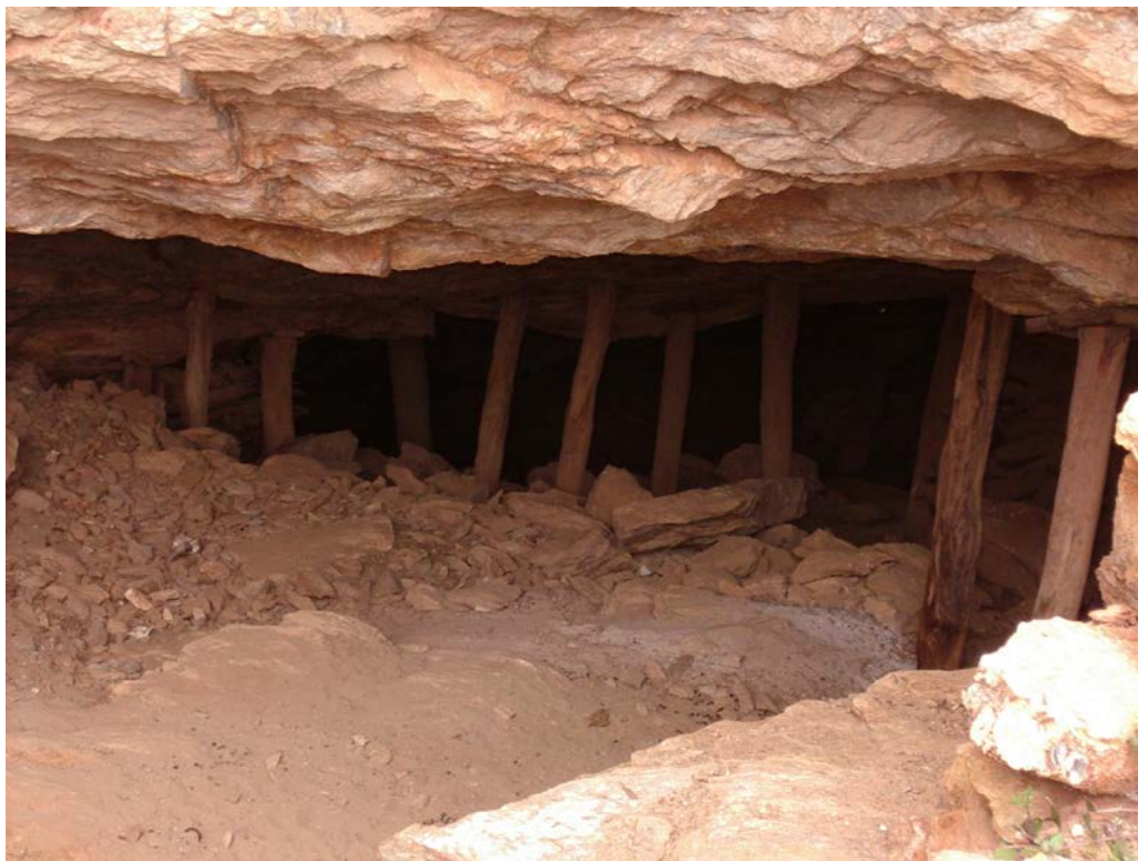
Top: Merton's Reward circa 1900. Fred Merton stands in front of a timber structure (a crib) supporting the roof (the back) of the underground workings. Bottom: circa 2004. These appear to be the same workings. The crib has been replaced with sturdy timber props. (Courtesy Navigator Resources Ltd, both images)
