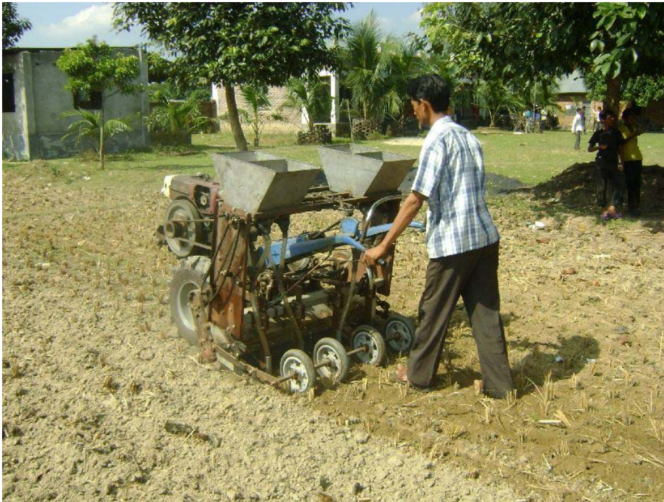
A locally made example of the ACIAR modified rotary tillage unit being tested in NW Bangladesh on October 2008
