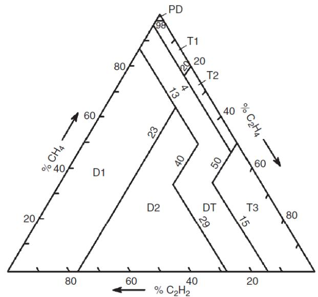
Fig. 2. Duval Triangle with fault regions [3], [4]
