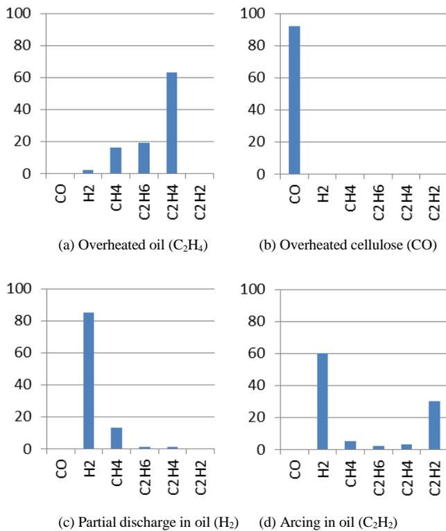
Fig. 1. Typical fault gas percentages (with their key gases) [1]
