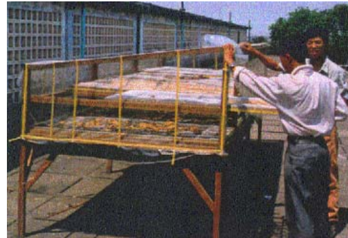
Fig. 1 Solar cabinet dryer [2].
