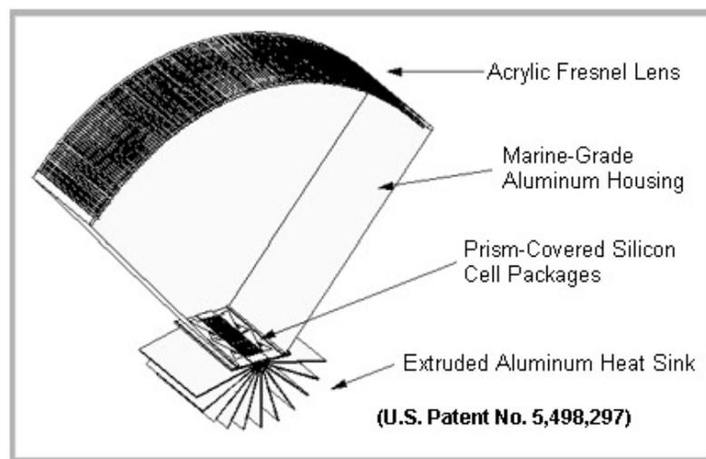
Figure 3.3.1 Module Cross Section
