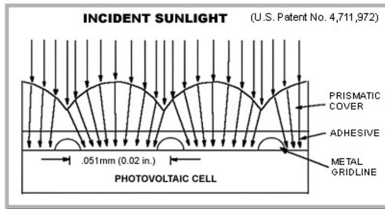
Figure 3.3.2 ENTECH's Prismatic Cell Cover
