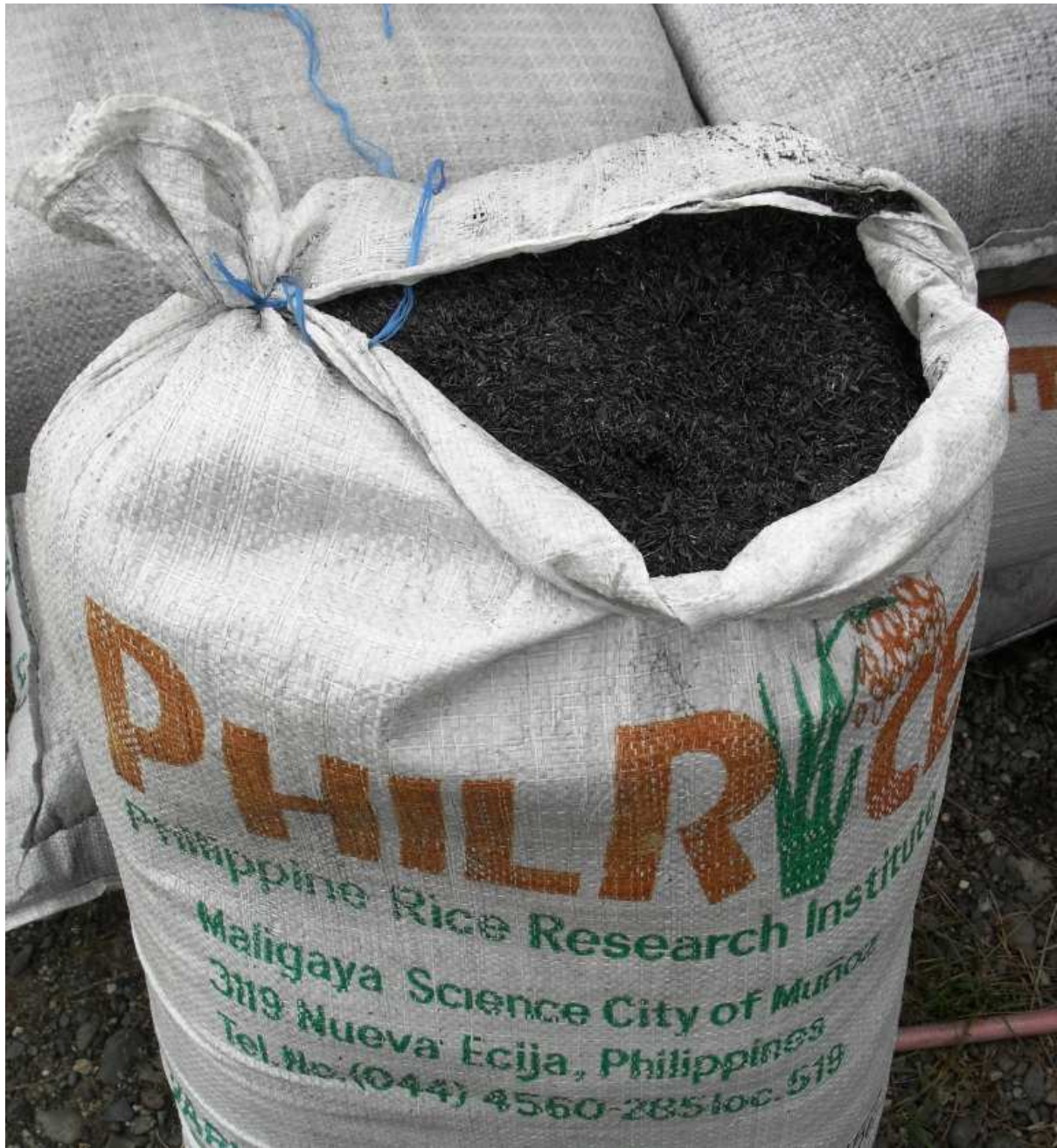
Figure 4 The bagged output biochar produced at PhilRice using the prototype carboniser, bagged ready for use in further experiments and organic fertiliser production.
