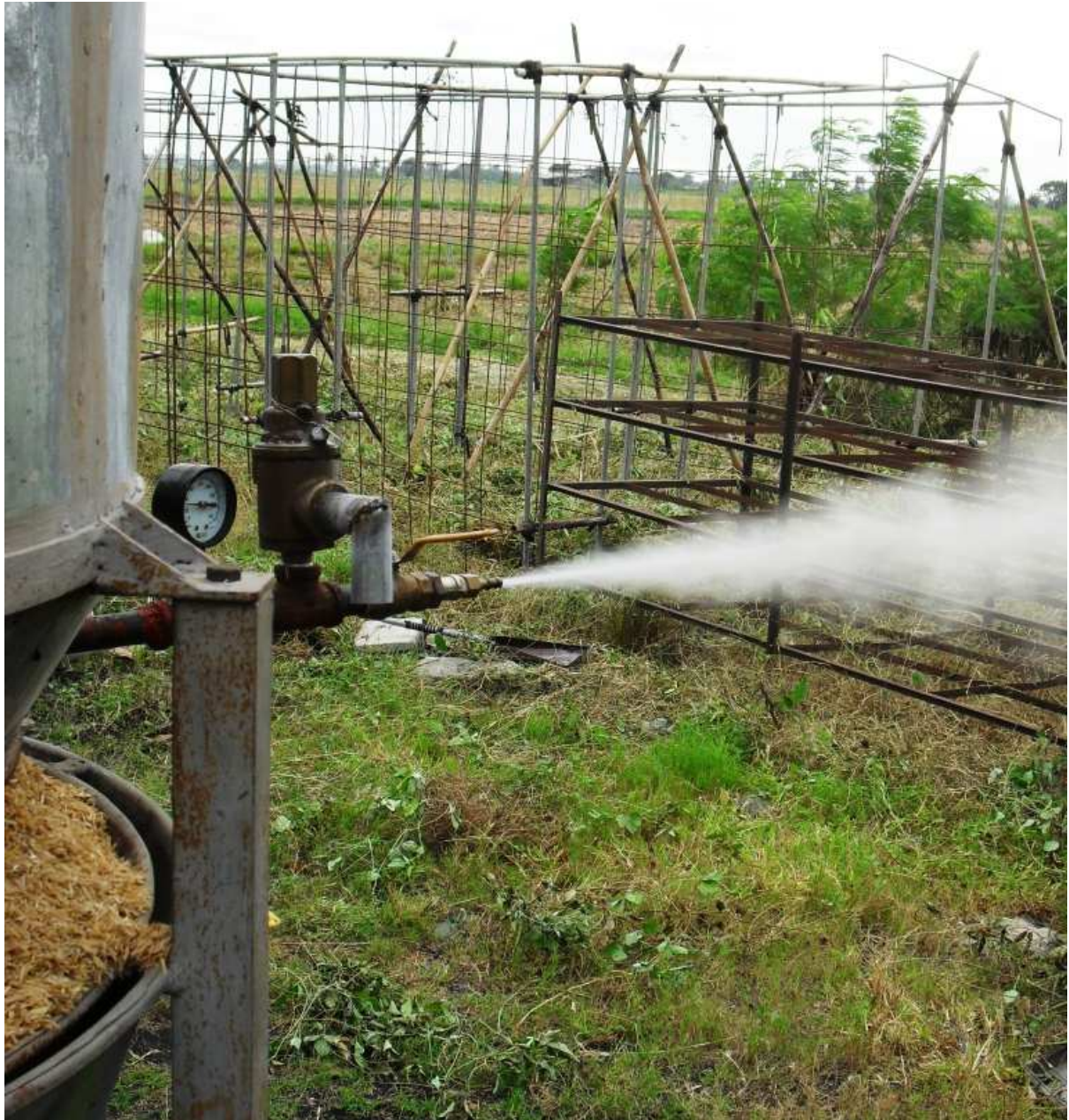
Figure 5 The carboniser retrofitted with an operational microboiler.
