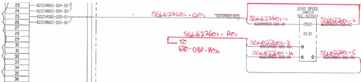
Figure 3: CEI Wiring Diagram for 240VAC Powered Instrument.
