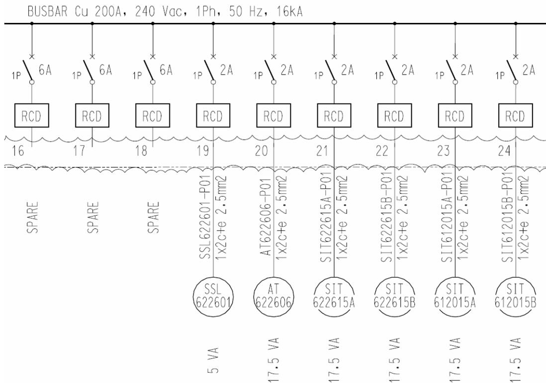
Figure 4: 620-DBP-704 Single Line Diagram.
