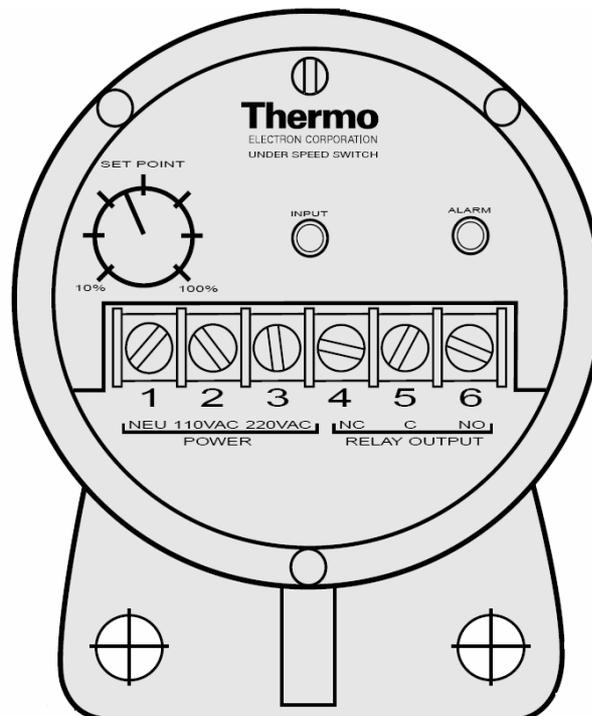
Figure 2: 240VAC Powered Instrument.
