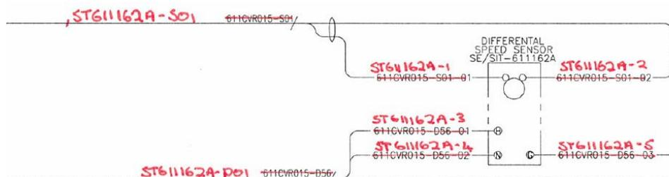
Figure 9: Mark Up of Cable Numbers
