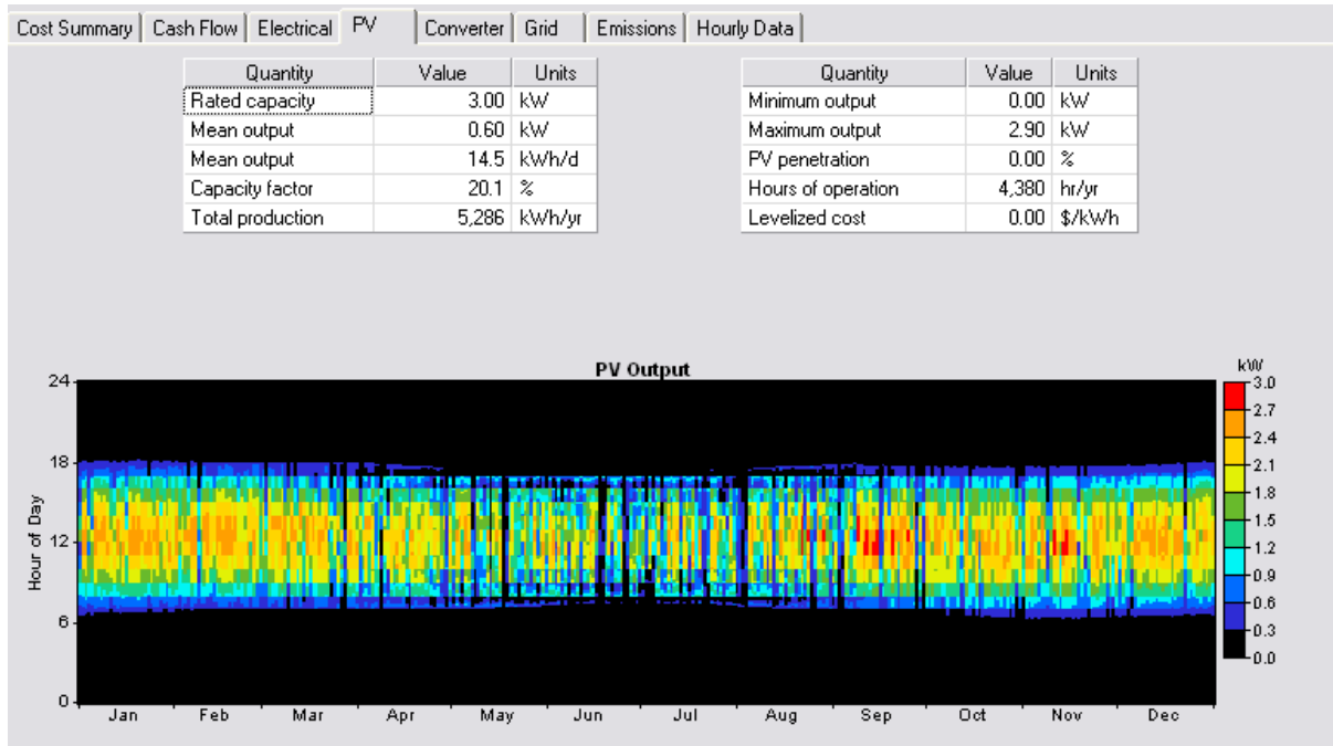
Fig. 6: Example 10 minute interval PV array simulated generation data for Perth.
