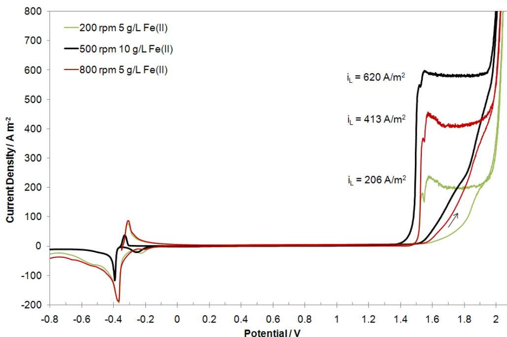
**Fig. 5** Voltammetric scans of a Pb-Ca-Sn anode in solutions of  $150 \text{ g L}^{-1} \text{ H}_2\text{SO}_4$  and  $5$  or  $10 \text{ g L}^{-1}$  iron(II) at various rotation speeds. The limiting currents shown are calculated from the Levich equation
