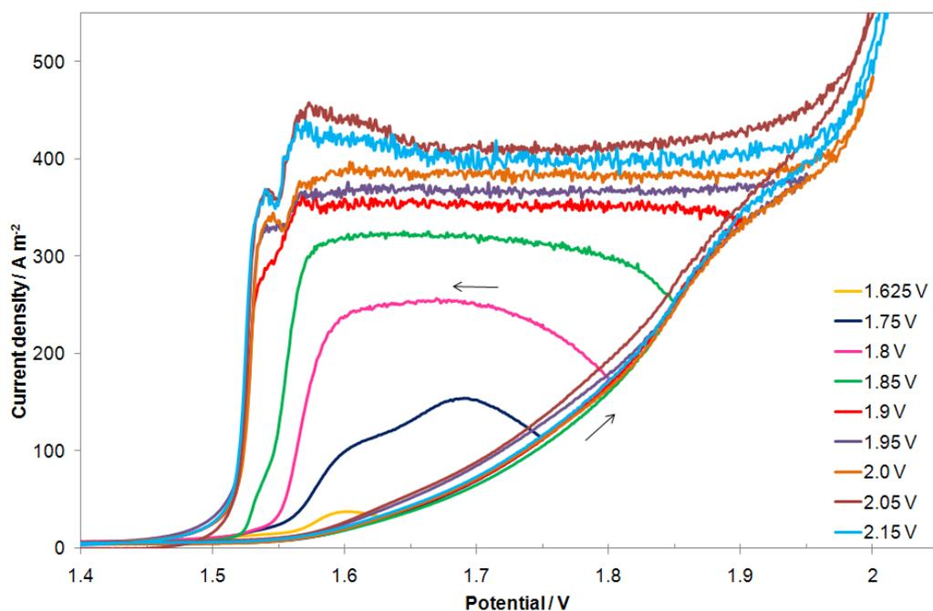
**Fig. 6** Voltammetric scans of a Pb-Ca-Sn anode in a solution of  $150 \text{ g L}^{-1} \text{ H}_2\text{SO}_4$  and  $5 \text{ g L}^{-1}$  iron(II) at  $800 \text{ rpm}$ . The positive potential limit was increased in successive sweeps
