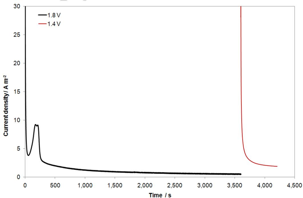
**Fig. 2** Current-time transients for the oxidation of a PbCaSn anode held at 1.8 V in a solution containing  $150 \text{ g L}^{-1} \text{ H}_2\text{SO}_4$  for 1 hour after which the potential was reduced to 1.4 V
