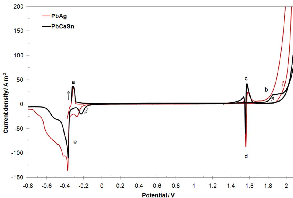
**Fig. 1** Voltammetric scans of Pb-Ag and Pb-Ca-Sn anodes in a solution containing  $150 \text{ g L}^{-1} \text{ H}_2\text{SO}_4$
