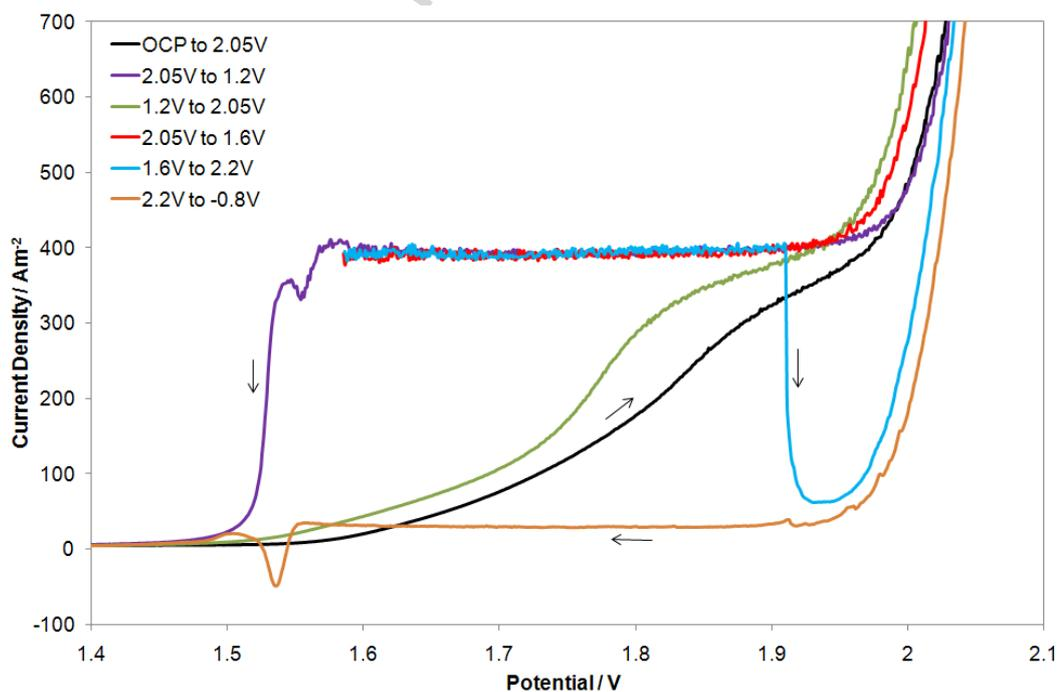
**Fig. 10** Successive voltammetric scans of a Pb-Ca-Sn anode in a solution of  $150 \text{ g L}^{-1} \text{ H}_2\text{SO}_4$  and  $5 \text{ g L}^{-1} \text{ iron(II)}$  at 800 rpm. Rotation speed reduced to zero at 1.9 V in penultimate sweep
