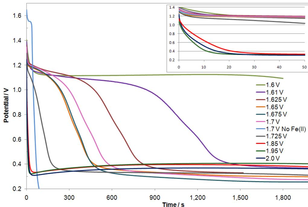
**Fig. 11** Open-circuit potential-time transients on a PbCaSn anode after oxidation at various potentials for 1 h in a solution of  $150 \text{ g L}^{-1} \text{ H}_2\text{SO}_4$  and  $5 \text{ g L}^{-1}$  iron(II) at 800 rpm. The curve at 1.7 V in the absence of iron(II) is also shown
