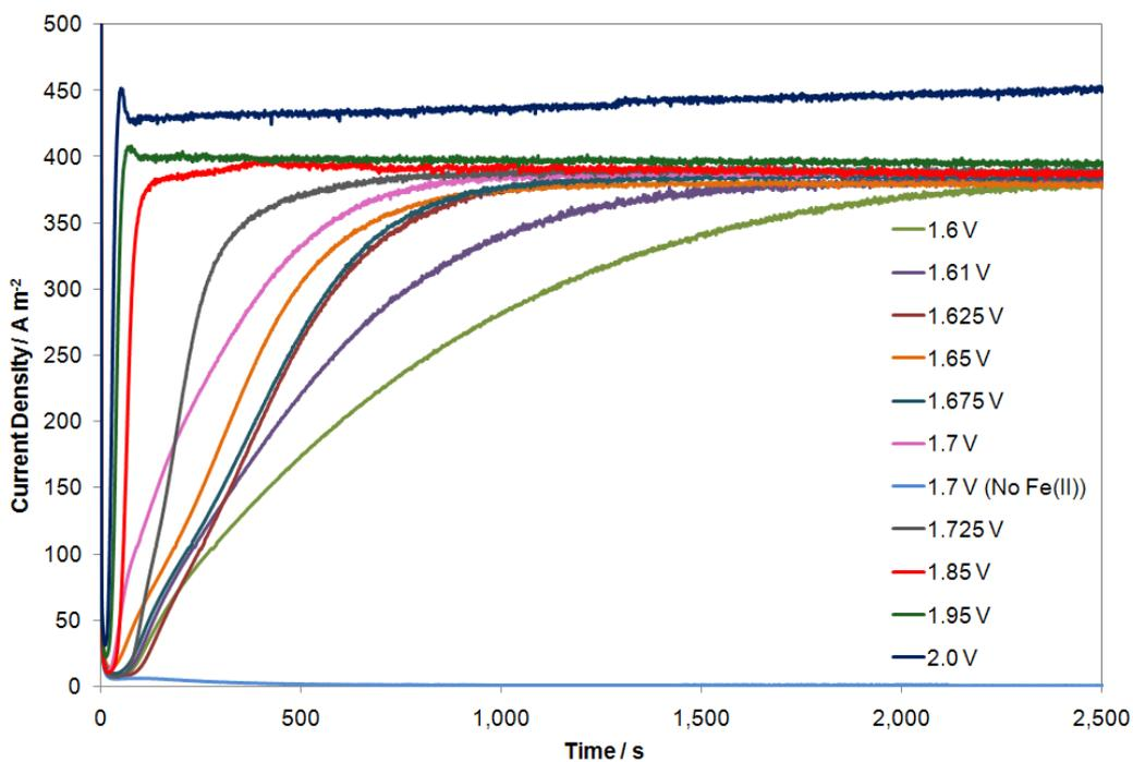
**Fig. 7** Current-time transients for the oxidation of iron(II) on a PbCaSn alloy anode held at various potentials in a solution of  $150 \text{ g L}^{-1} \text{ H}_2\text{SO}_4$  and  $5 \text{ g L}^{-1}$  iron(II) at 800 rpm
