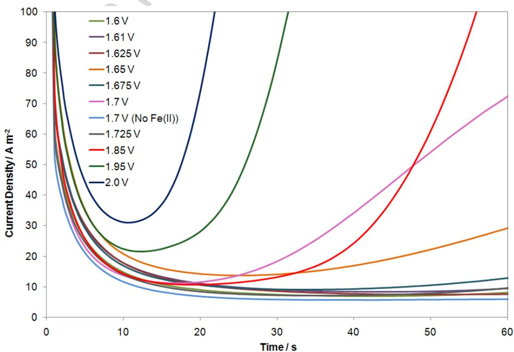
**Fig. 8** Current-time transients for the initial stage of oxidation of iron(II) on a PbCaSn alloy anode held at various potentials in a solution of  $150 \text{ g L}^{-1} \text{ H}_2\text{SO}_4$  and  $5 \text{ g L}^{-1}$  iron(II) at 800 rpm
