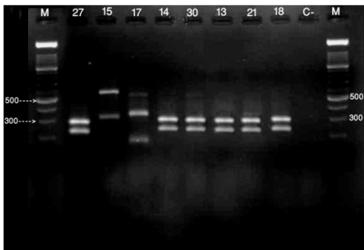
Fig. 2: Patterns of PCR products of Candida isolates after digestion by the restriction enzyme MspI . Lanes of 27, 14, 30, 13, 21 and 18 represent C. albicans ; 15, C. glabrata and 17, C. guilliermondii . Lane M is 100 bp ladder molecular size marker and C is negative control
