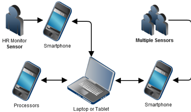
Fig. 3. Device topology in a mobile simple usage scenario
