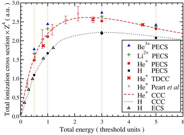
FIG. 1. TICS calculations for  $Z \leq 4$  targets at total system energies of 0.5, 1.0, 3.0, and 5.0 t.u. The energies of our PECS calculations are indicated by vertical dashed lines. Comparison is made with ECS [8] and the  $l_{\max}=4$  CCC calculations of Ref. [17] for H; CCC [11], TDCC [13], and experiment [18] for  $\text{He}^+$ . All TICS have been multiplied by  $Z^4$ .
