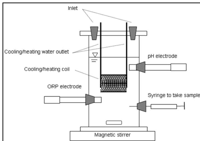
**Figure 1.** Batch reactor.
