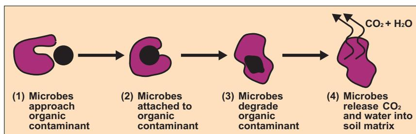
Figure 3: Mechanisms of bioremediation (Adapted from USEPA, 2001)
