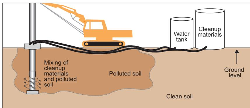
Figure 4: In-Situ solidification/stabilization of contaminated soil (USEPA, 2001)
