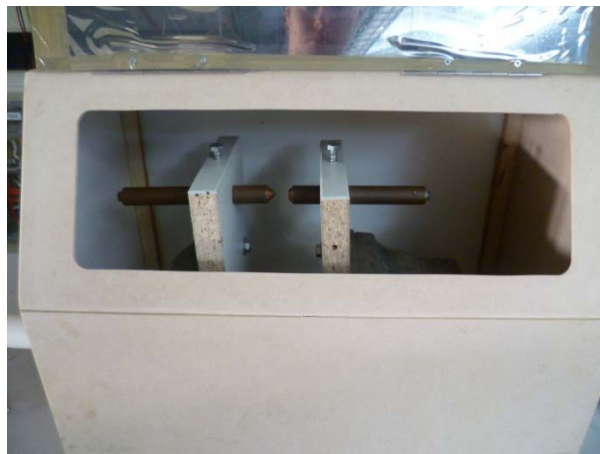
Figure 9 Arc creation device enclosed for additional safety
