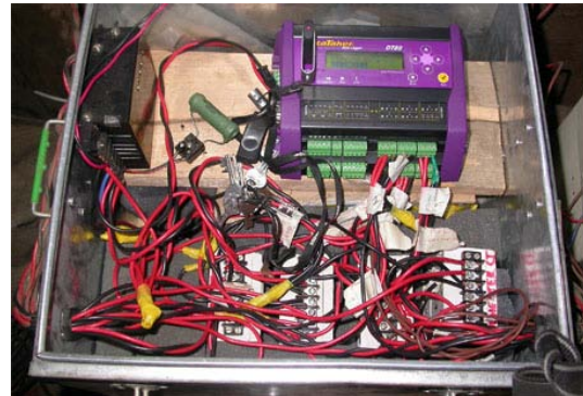
Figure 6: A sophisticated dataTaker DT80 data logger monitors and records 22 different parameters for one of each of the three types of solar PV village systems RDIS-Nepal developed. This provides us with detailed data for long-term performance.
