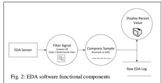
Fig. 2: EDA software functional components
