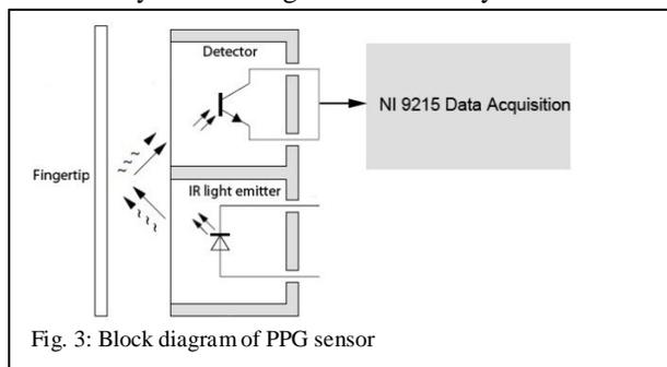
Fig. 3: Block diagram of PPG sensor
